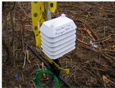
Fig 3. A) Burkard Spore trap. B) Watchdog weather station monitoring soil moisture, soil and air temperature, and relative humidity.
