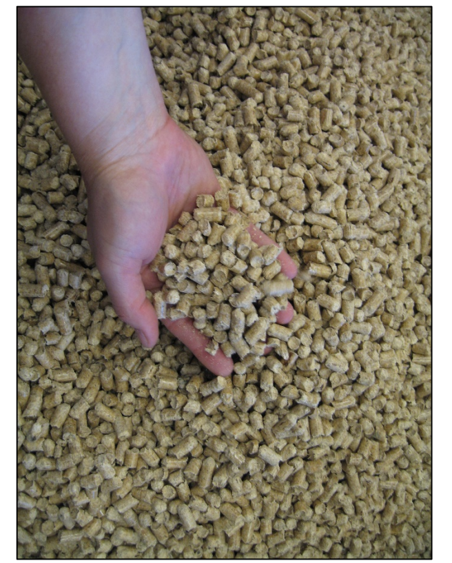
Pellets must be uniform in size and quality to ensure trouble-free automation of household heating systems.
