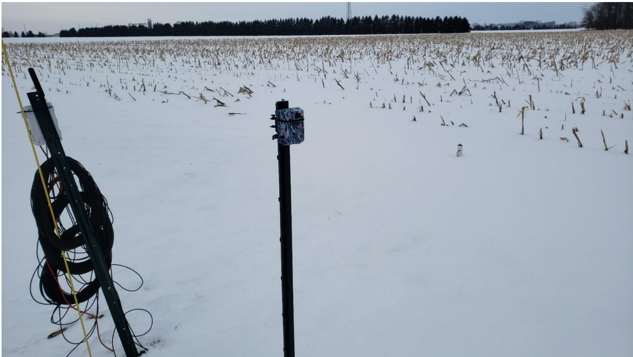
Figure 2 - Browning Trail Camera that was used for observing surface runoff. This camera is located at the BL site.
