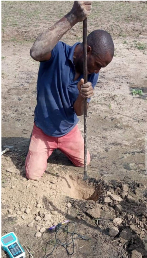
Taking soil samples at lower depths. Digging through hardpans
