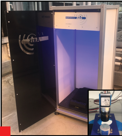
Fig. 1. Aris Top View Image Station where leaf area of plug trays was estimated non-destructively.
