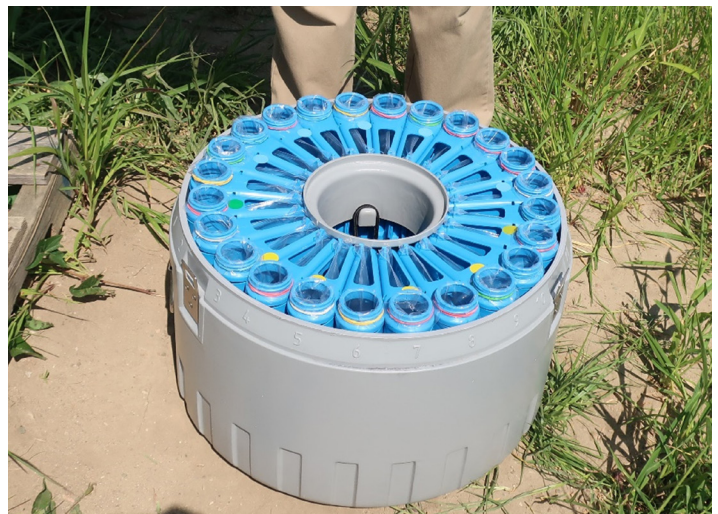
Figure 1- An automated sampler can perform flow-proportional or time-proportional sampling.
