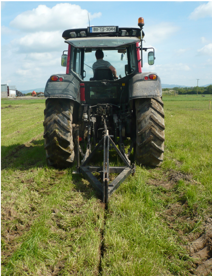
Figure 4- A tractor pulling a mole plow. The shank creates a blade-cut to break up the plow-pan and compacted surface layer to improve infiltration and aeration (Photo credit: Patrick Tuohy).
