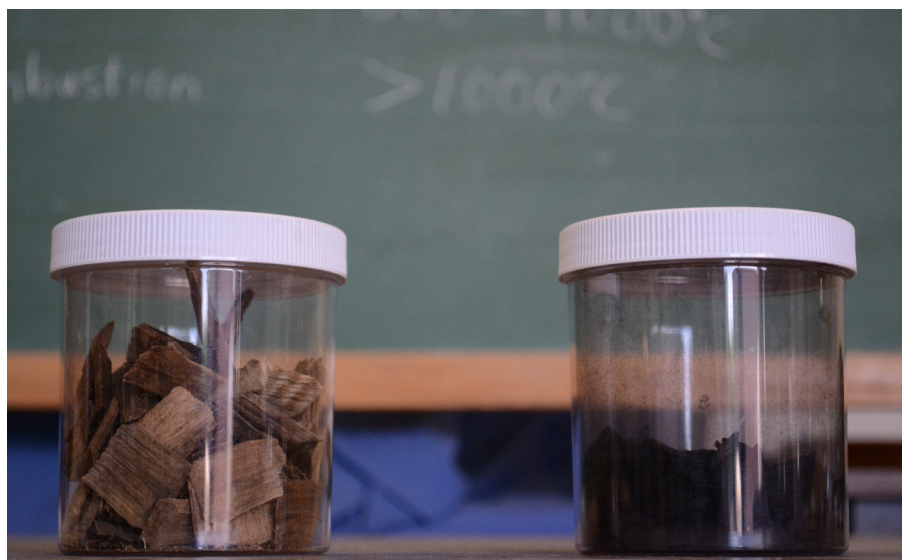
Torrefaction converts woody biomass (left) into a solid, dry, brittle and blackened material called torrefied biomass, or bio-coal (right). Photo provided courtesy of Dr. Saffron.
